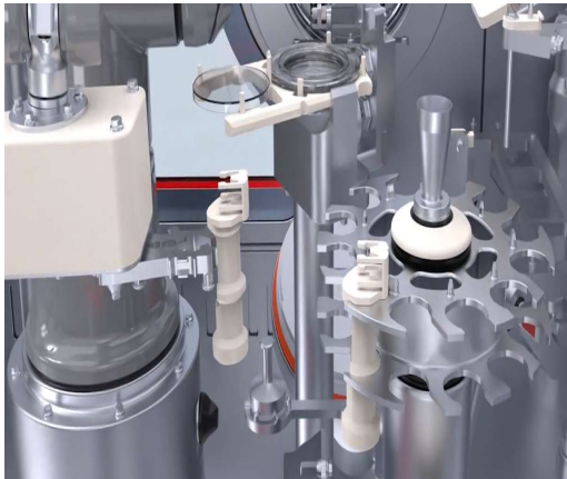
Installation of autoclaved format size parts
