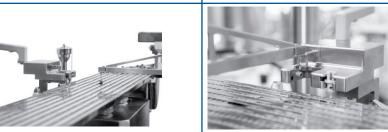
co Camera detects the incorrectly sorted stopper and it's individual position by using AI in the short linear track
