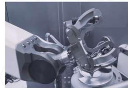
Specific design and development to open the crimp of the aluminum
