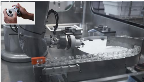
#5 Place vial on rotary table
