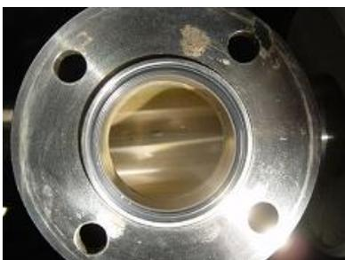
CO<sub>2</sub> trap shouldn't be allowed to collect moisture as this can cause blockage.
